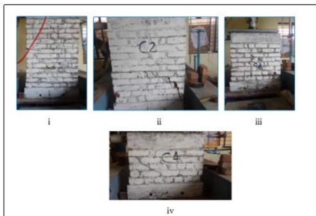
Fig.4 failure pattern of burnt clay hollow brick wall of aspect ratio i)1.234 ii)0.99 iii)0.713 iv) 0.444
